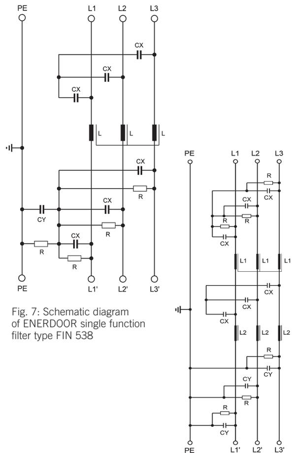
Fig. 7: Schematic diagram of ENERDOOR single function filter type FIN 538
