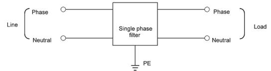
Fig. 5: Schematic diagram of a single phase filter
