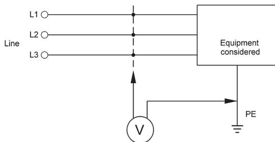
Fig. 2: Common Mode Interference
